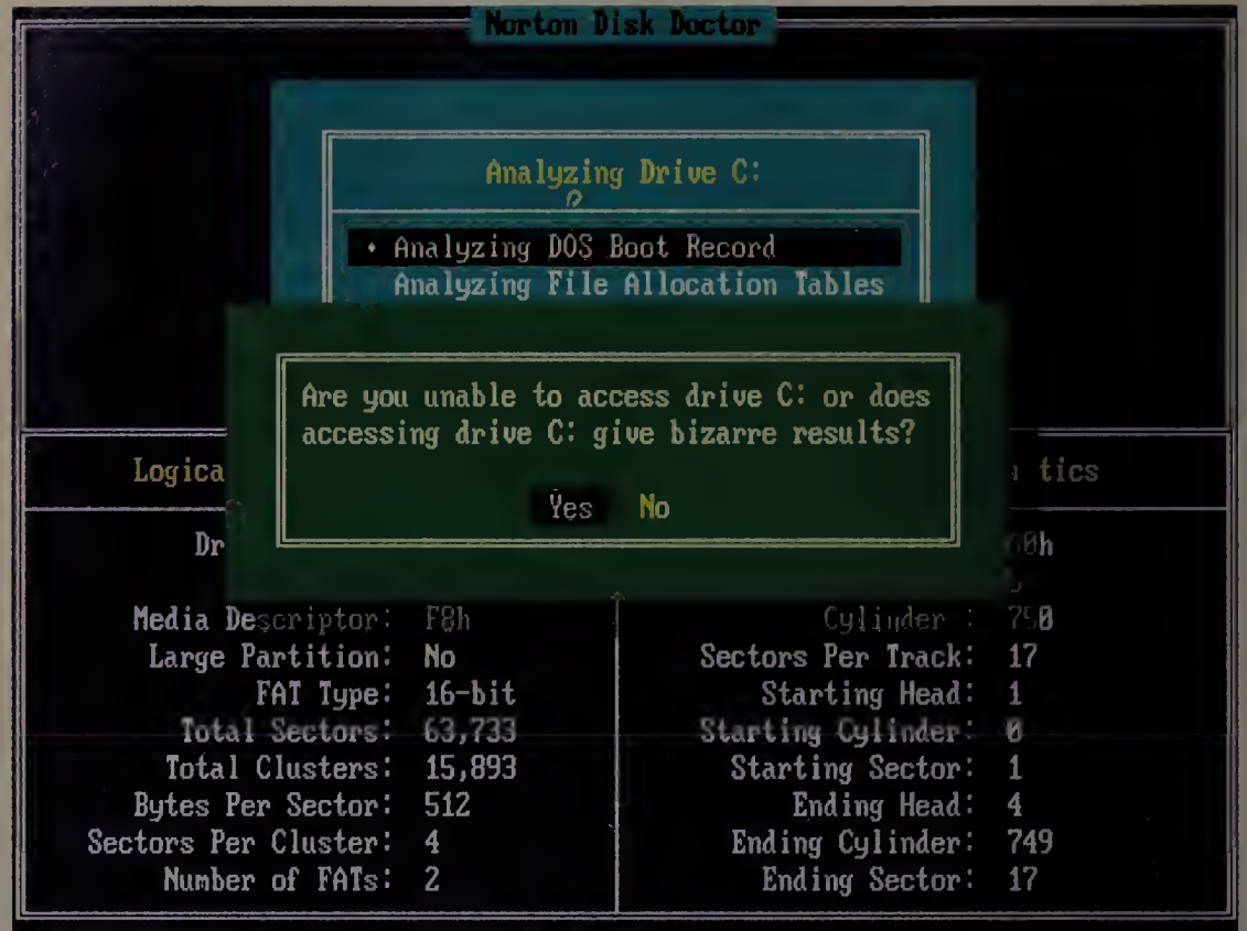
Norton's Disk Doctor displays its friendly bedside manner when it detects damage to a drive's boot area.
